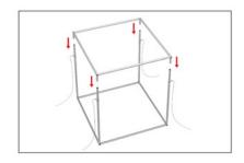
A Slide cable loop onto the end of corner before attaching. B Screw eyebolts into corners and before attaching. attach cables.
